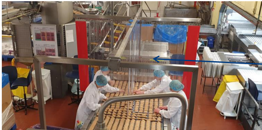
Perspex screens on cake manufacturing line to ensure colleague safety
